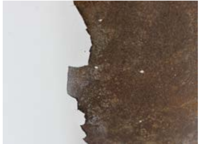
Fig. 7: Rust in area of paint delamination.
