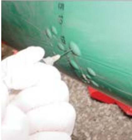
Fig. 4: Solution extraction for laboratory analysis; high alkalinity solution was present in the blister.
