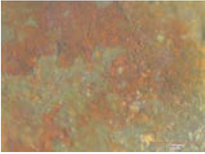
Fig. 8: Photomicrograph of rust on underside of primer at 7-times magnification.
